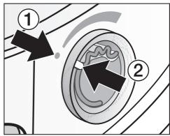
■ Turn the outer ring anti-clockwise until markers ① and ② line up.
